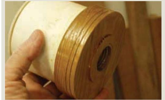
Bottom view of completed vacuum chuck.
