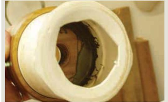
Top view of completed vacuum chuck with gasket in place.
