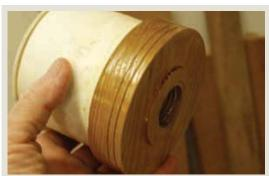
Bottom view of completed vacuum chuck
