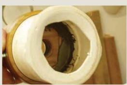
Top view of completed vacuum chuck with gasket in place
